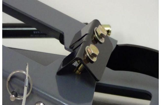
Top Head Lock Bolts Loosened
