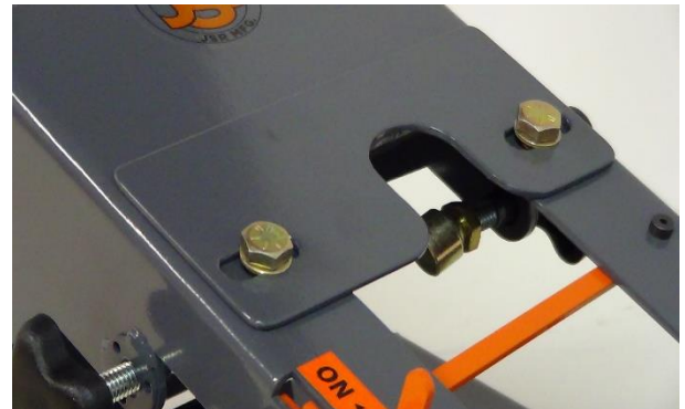
Top Adjuster Plate Bolts Loosened
