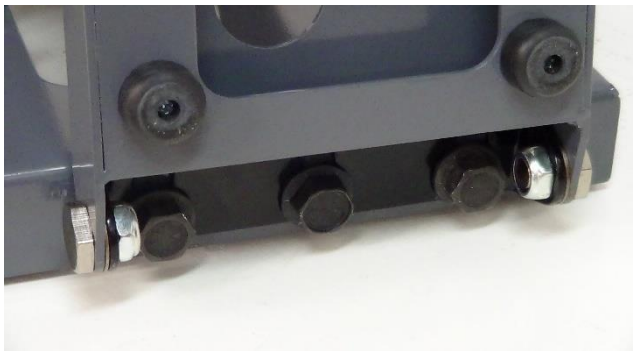
Three (3) Base Hinge Loosened
